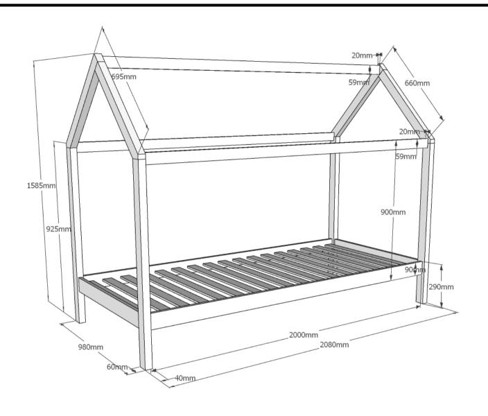
L:2080mm H:1585mm D:980mm innersize 900x2000mm
