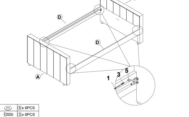
STEP 3:At the back, install the backrest (part (a)) by using hardware provided, use Allen key part (a) to screw in the bolt (part (a)) and washer (part (b)) on each side (2 bolts & 2 washer on each side).
