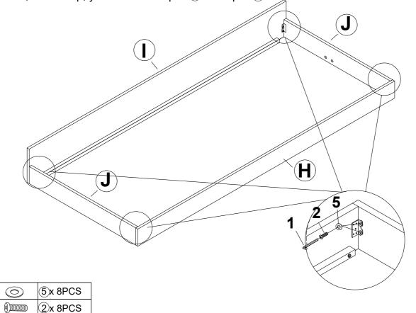
STEP 7: This step is similar to step 4, you will need 4 part(5) & 4 part(2) and screw in the bolts to the trundle side panel.
