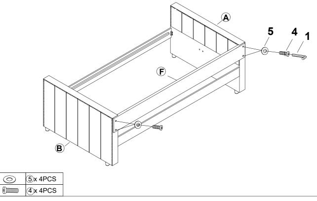
STEP 4: Take the upper support bar and lay it in the middle of the Bed from left and right armrest, you will need 4 part 3 and 4 part 5 to screw in the bolts to the Armrest.
